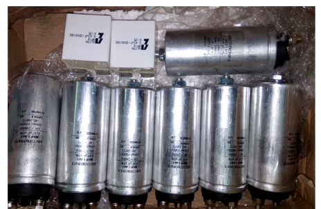
SNUBBER & START CAPACITOR
